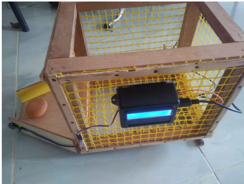
Figure 7. Final Prototype to measure the pawing frequency of laying hens.
