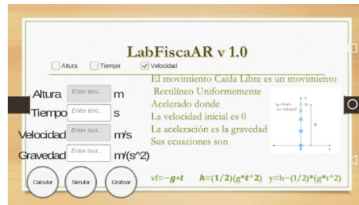
Figure 6. Free Fall Interface. Illustrates a definition and the equations that are involved in the free fall movement, allows to perform calculations knowing two of the variables that intervene in the equations
